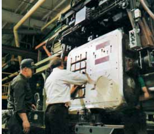
(Right) A machine operator at a plastics manufacturer removes a thermoformed shipping container for automobile headlights from a rotary vacuum press.
